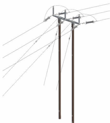
Typical Trident angle pole with stays
